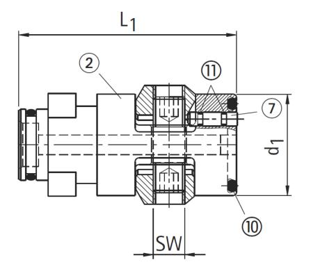
Used for the application with coolant pressure up to 150 bar suitably.
