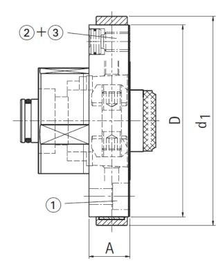
Used for fitting onto machine spindle for holding HSK tools.
