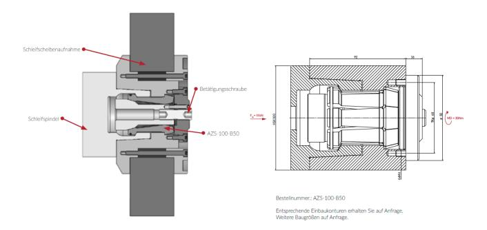
The AZS gripper is specially designed to manually mount heavy grinding wheels to a standard HSK 100 tool interface.
