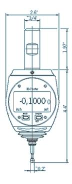
The Digital 3D-Sensor is a further development of the time proven Mechanical 3D-Sensor. It serves for approaching workpiece edges on milling and EDM machines. The spindle may be positioned quickly and safely on the references edge. The approaching operation can be exactly monitored on the digital display. The 0-position is found on the first try. The machine coordinate system can be set without any calculations because the spindle axis is positioned exactly on the approached edge.
