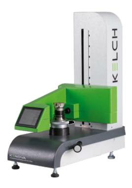
The next stage up is the KENOVA Setline V466 with its greater measuring range: 600 mm diameter and 600 mm in length. The Setline V466 shines out among the competition thanks to its modern and ergonomic design as well as to some adjustment related to current market demands. The SK50 precision spindle with vacuum and spindle clamping, mounted on an anti-friction bearing, lays the foundation for precise measurements.
