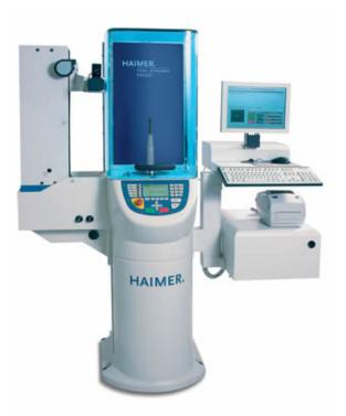
Balancing and presetting are key elements of modern manufacturing. It is obviously a good idea to combine these two procedures. The Tool Dynamic Preset is a perfect combination of Haimer's balancing technology and Zoller's measuring technology. The tool is clamped in the high precision balancing spindle fitted with Haimer's proven adapter system. This saves time and increases accuracy because the tool does not have to be re-clamped.
