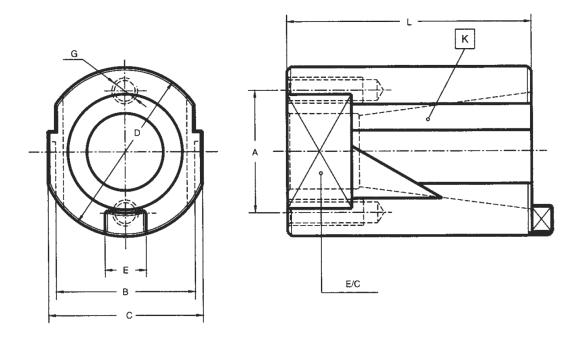
The Basic Mounting Fixture is a simple yet effective way to work with your tool holders. The fixture is designed for mounting or simply holding in a vise. Additionally, in conjunction with a surface plate and height gauge, the mounting fixture can be used as an inexpensive alternative to a presetter.
