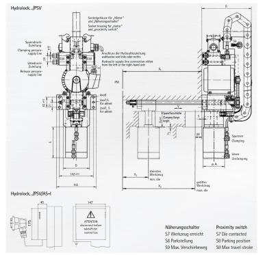
The drawbar style hydromechanical (hydrolock) self-locking die clamping system is designed for clamping dies of various widths on press slides. The clamping actuator moves automatically in the T-slot of the press slide between the parking position and the respective die. Clamping and unclamping are performed by a hydromechanical self-locking clamping gear. Hydraulic pressure is at a maximum 90 bar.
