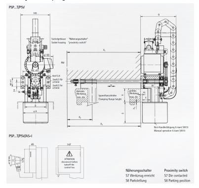
The mechanical disk-spring washer style die clamping system is designed for clamping dies of various widths on press slides. The clamping actuator moves automatically in the T-slot of the press slide between the park position and the respective die. Clamping is performed by belleville spring washers and hydraulic unclamping.
