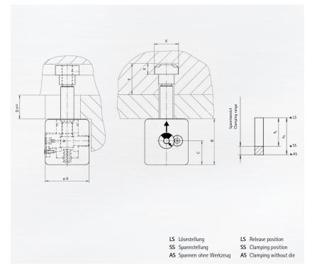
The manually actuated drawbar style die clamping system is designed for clamping dies of various widths on press slides and tables. The self-locking eccentric cam gear guarantees a simple handling with a maximum of safety.
