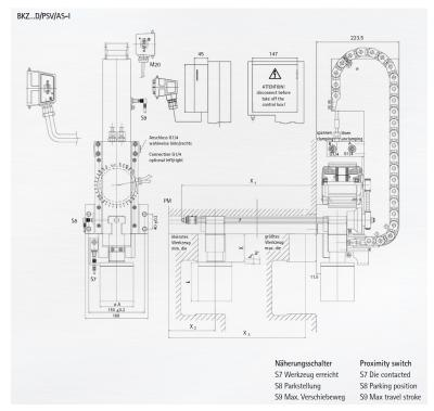
The hydraulic die clamping system with drawbar style clamping is designed for clamping dies of different widths on press slides. The clamping actuator moves automatically into the T-slot of the press slide between the parking position and the respective die. The clamping element can clamp different clamping rim heights due to the long clamping stroke of the double acting cylinder. Hydraulic pressure is at a maximum 400 bar.
