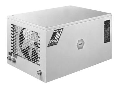
The unit comes complete with a powerful water pump, tank, and complete electric controls. The uniquely designed evaporator allows water inlet temperatures down to 2° C without the use of frost inhibitors. Even freezing will not damage or cause the unit to fail. By using a BKW re-cooling unit, ever increasing cooling water costs can be avoided.
