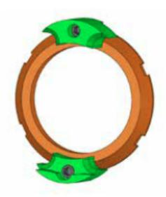
Can be mounted in front of the spindle shaft after the installation of the collet. Has the advantage of being adaptable to HSK-E or HSK-F tool interfaces in an HSK-A spindle. Just use the drive key to expand and then clamp the desired tool. The ENS slot nuts can also be used in manual clamping units for more flexibility. Available for HSK 32, 40, 50, 63, 80, and 100.
