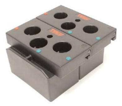
The tool carrier measures 240 x 120 x 130 mm and has 2, 3 or 5 locations for holding tools with a tapered or cylindrical shank. The plastic used is shockproof and resistant to all substances which are usually present such as oils, fats, petrol.
