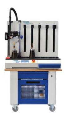
The Power Clamp Premium/Premium Plus is the shrink fit machine for perfectionists. The cooling bodies are fixed at linear guides. For the cooling process they are exactly centered put on the hot shrink fit chuck. The cool down phase is terminated temperature controlled automatically.
