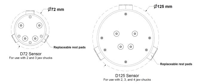
The ForceCheck wireless chuck force gauge is designed to quickly and accurately measure holding force and speed on chucks. Verifying chuck holding force allows manufacturers to improve the repeatability of a manufacturing process by checking actual holding force under dynamic (rotating) conditions, as well as perform critical preventative maintenance checks.
