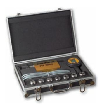
Enables quick and simple measuring of pressure and rate of flow of coolant when the actual tool is clamped directly in the stationary tool spindle. This way, it is possible to establish the real conditions of the relevant machine and tool configuration and measure the resulting actual rate of flow.
