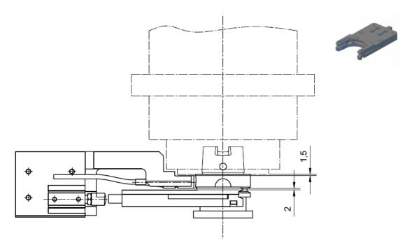
The locking gripper offers the same features as the heavy duty gripper, but adds the benefit of a locking mechanism to retain the tool. Because the tool cannot be removed from the gripper, this design is ideal for rapid acceleration or extremely heavy tools. Unlocking can be mechanical, electric, or pneumatic depending on customer requirements.
