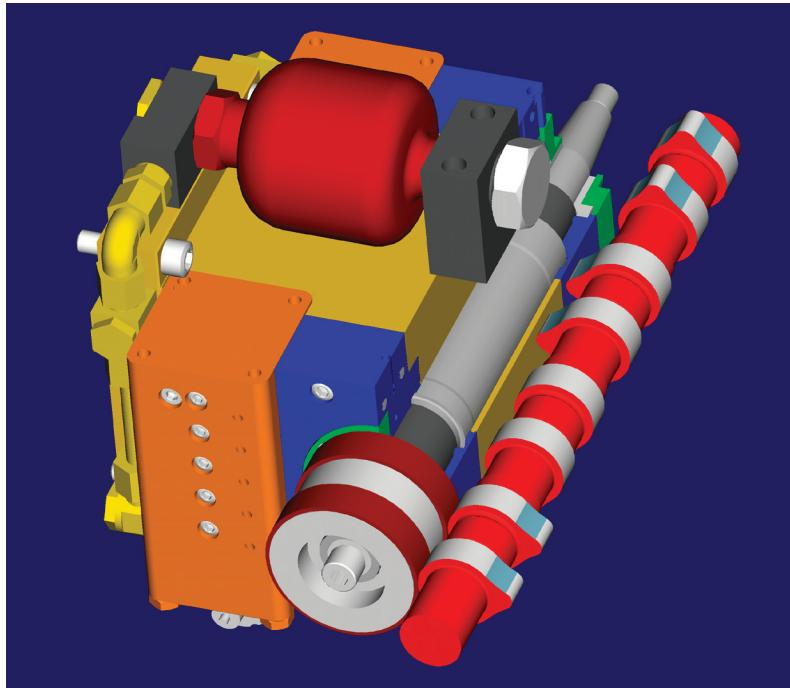
This is an example of a hydrostatic spindle designed for high speed grinding with CBN grinding wheels. The small bearing diameter in combination with high surface speed allows the use of CBN wheels even for undercuts in a camshaft application.
